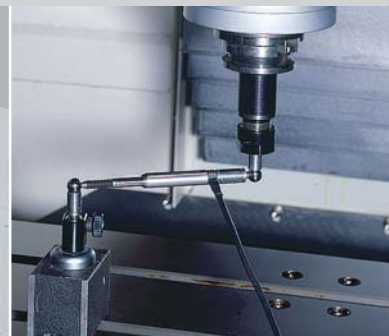
The Renishaw ball bar instrument calibrates the circularity and the geometrical accuracy to ensure precise three-dimensional motions.
